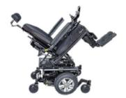
Electronically powered wheelchair. Features may include seat elevation, tilt, recline, powered elevating leg rests, joystick controller, Chairs can have either front, mid, or rear wheel drive.
